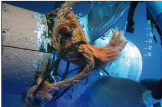
Rope and cable found wrapped around the propeller of the Esperanza of the Greenpeace fleet, off the coast of St Helena, South Atlantic, 7 March 2006 © Greenpeace/Dave Walsh
