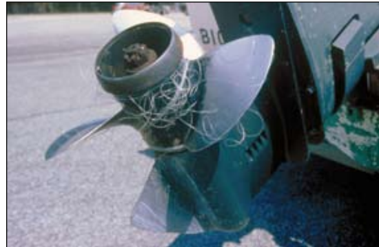
Nylon fishing tackle entangling an outboard motor propeller.
